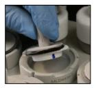
9. After the 1 minute re-cooling, attach the chuck in its cryostat housing in the same position used for the trimming.
